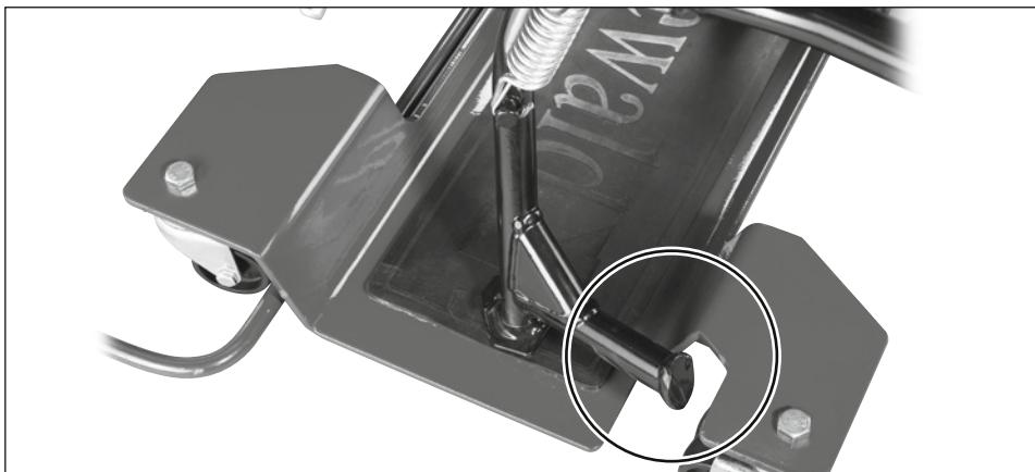
Push the Bike Mover under the motorcycle at a 90° angle, from the left side of the bike, so that the centre stand can rest on the metal platform. Make sure that the lever of the Bike Mover's parking brake is pointing towards you. The foot pedal on the centre stand must not impede the lever, and must not rest on the edge of the wheel plate. Otherwise the motorcycle will not stand firmly and may topple over. Try this out with special care when you use the Bike Mover for the first time. When you're
