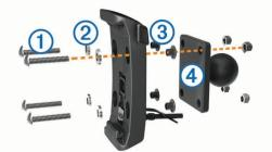
2 Tighten the nuts to secure the base plate.
