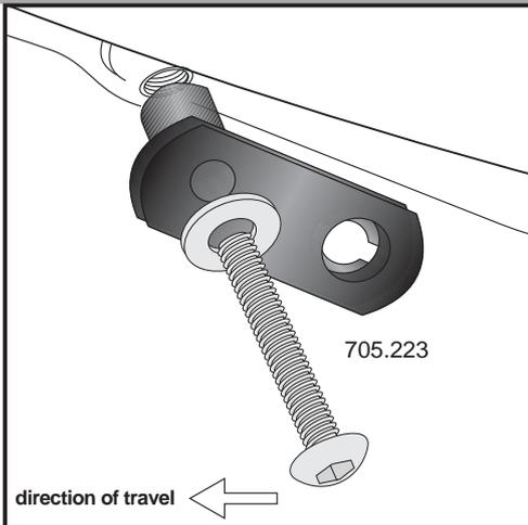
**4** Fastening of mounting strut 3 and 4 above left + right:
