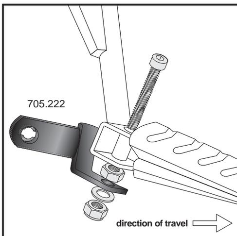
**3** Fastening of mounting strut 2 front right:
