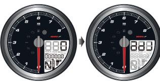
•When the engine switch is OFF, hold the **button for 3 seconds** to enter settings.
