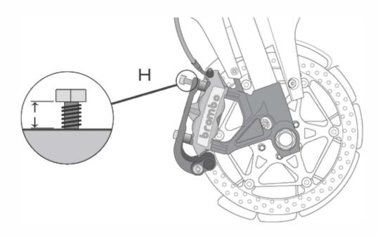
**NOTE 1:** If proper installation requires a thread length in between 80mm and 90mm, the included 5mm shims (X) can be used between the bolt and the RoadLoK body. Combining the 5mm shim with the 90mm bolt will result in an effective 85mm thread length, which may be more appropriate for some models.
