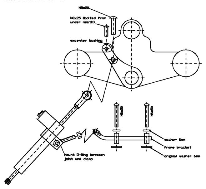
Steering damper is designed to be mounted on left side of the fuel tank parallel to left handle between handle and tank.
