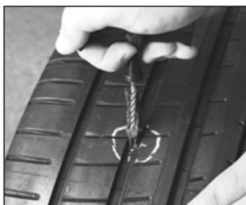
Insert the repair string into the puncture using the repair tool, allowing it to still protrude at least 13 millimetres.
