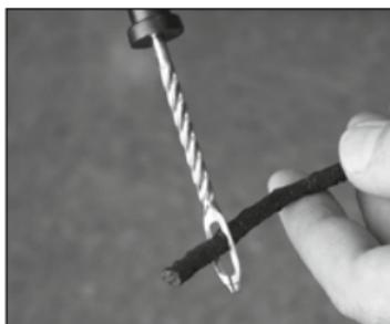
Peel off a sealing strip from the protective film and insert it into the needle eye of the repair tool.
