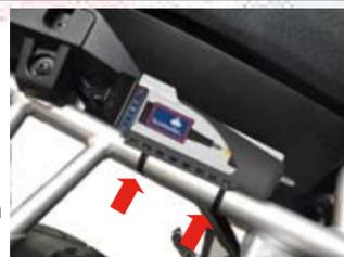
Route the vacuum tubing to the top of the RMV. Trim and save any offcut. Push the end of the vacuum tubing into the top of the RMV.
