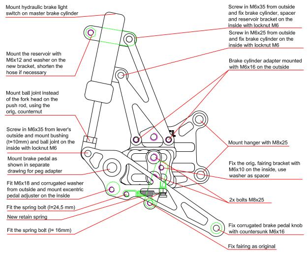
Advice: The orig. bracket for brake cylinder and brake light switch is inapplicable! Use the attached bolts M8x40 for threads M8 and M6x35, with the rubber coated clamp to guide the wiring harness, for the upper thread M6
