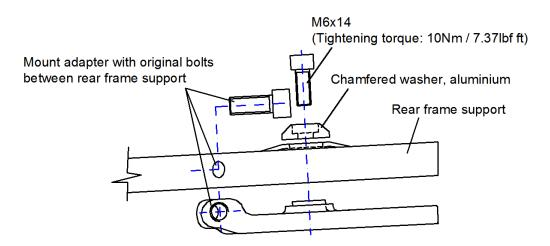
Equip new frame cover with taillight and flashers (not included), then mount rear frame cover tension free.
