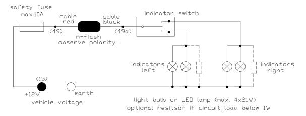
ATTENTION! THE MINIMAL SUPPLY CABLE WIDTH IS 0,75MM<sup>2</sup>. YOU MUST FUSE THE +12V POWER SUPPLY CABLE WITH A 10A SAFETY FUSE. IF THE DEVICE WILL BE USED WITHOUT FUSE, DAMAGE AT THE CONNECTING CABLE OR THE M-WAVE ITSELF CAN CAUSE A SHORTCUT AND A CABLE FIRE. THERE MAY BE A RISK OF YOUR LIFE! IF YOU ARE NOT CAPABLE TO CONNECT THE DEVICE PROPERLY, LET THE PROFESSIONAL MOTORCYCLE TECHNICIAN DO THE JOB.
