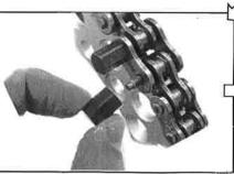
**®**Tighten the right and left nuts with a wrench (10mm) by rotating 60° alternately to press the outer plate into the pins.
