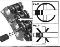
(4) Screw the nut again at the point of Fg. 3. Hold the nut with the wrench and snap off the pins.
