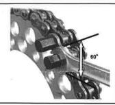
(13) Remove the nuts and check that the outer plate is completely pushed as shown Fg. 1.
