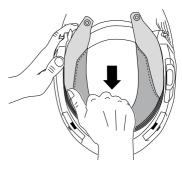
**2.** Attach the plastic hooks between the helmet shell and the lining
