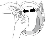
**3.** Relocate the neck pad onto its fixing between the helmet shell and lining, and do up the buttons on the front tab of the neck pad.
