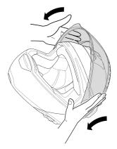
**3.** Check the function of the visor mechanism by closing the visor once and opening it as far as possible.
