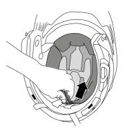
**2.** Undo the two buttons in the forehead area and remove the head padding.
