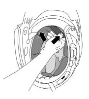
2. Insert the plastic retention flaps with round holes over the pins sewn into the rear section of the cheek pad and affix them using the red snaps.
