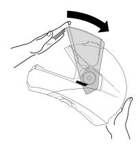
2. Press the spring underneath the face shield mechanism on one side towards the face shield opening, then do the same with the spring on the other side.
