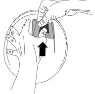
2. After cleaning, re-attach the ventilation cowl by sliding it into the mechanism and applying pressure until it clicks back into its original position.
