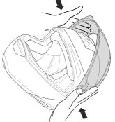
2. The face shield will then audibly lock into place when you press it gently towards the helmet with a simultaneous closing movement.
