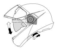
The maximum opening position of the sun visor can be set in a choice of two latched positions using the limiter. The limiter is on the running edge of the sun visor slider.
