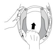
2. Undo the plastic hooks between the helmet shell and the inner lining on the front tabs of the neck pad.
