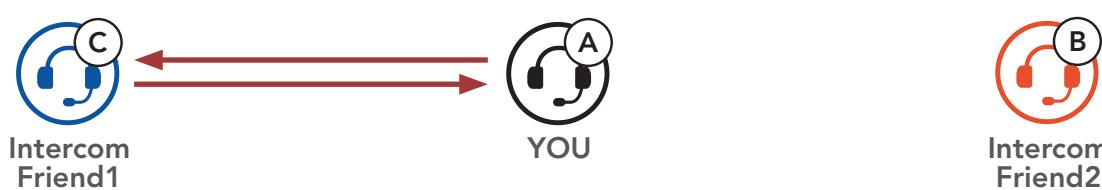
3. You (A) can call the **Second Intercom Friend (B)** by double tapping the **Center Button**, or the **Second Intercom Friend (B)** may join the intercom by making an intercom call to you (A).
