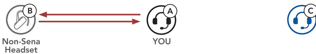
3. The other Bluetooth system (**C**) may join the intercom by making an intercom call to **you (A)**.
