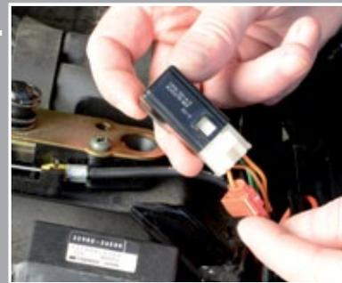
Remove switched positive (ignition) from starter relay
