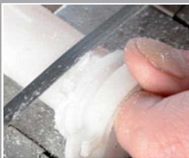
Carefully saw off protrusions on throttle tube...
