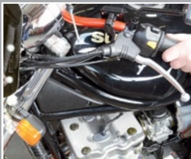
**20** Fix switch to handlebar or controls.
