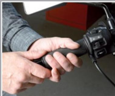
install grip with cable outlet facing down.
