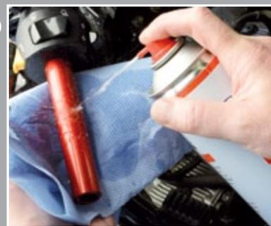
Degrease and clean left end of handlebar.
