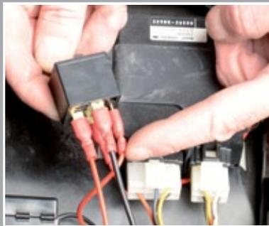
Use insulated cable terminals for connection.
