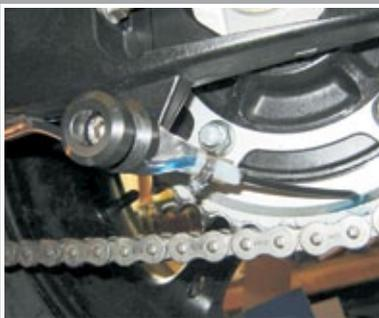
Install the oil injector nib and oil tube
