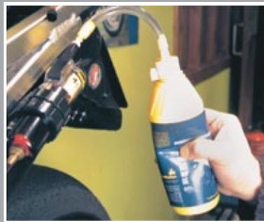
Remove air bubbles and bleed delivery tube
