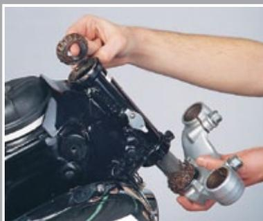
Grease well, assemble and adjust
