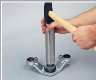
Drive in taper roller bearing
